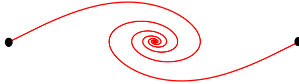
FIGURE 3. The Birkhoff attractor for the pendulum with friction
